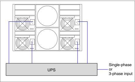
Figure 72: Single basic unit with a single UPS
